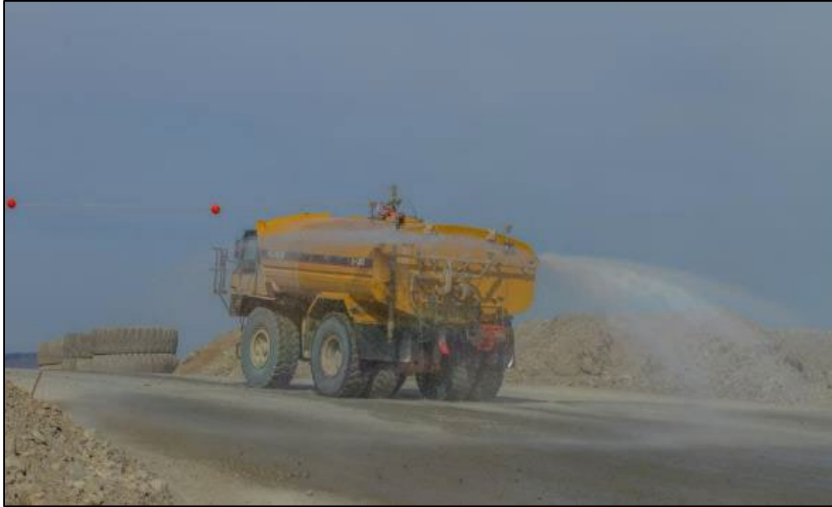
FIGURE 3.18: WATERING HAUL ROADS WITH 13,000 GAL CAT 773 WATER TRUCK.
